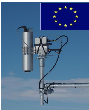
HYPSTAR® system [https://hypstar.eu/] 380-1700nm, 3-10nm FWHM
