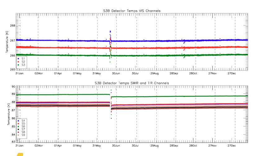
SLSTR-B detector temperatures for each channel from Jan 2022 to end of Jan 2023. The discontinuity in the IR channels in June 2022 is a result of the anomaly and subsequent decontamination. The vertical dashed lines indicate the start and end of each cycle.
