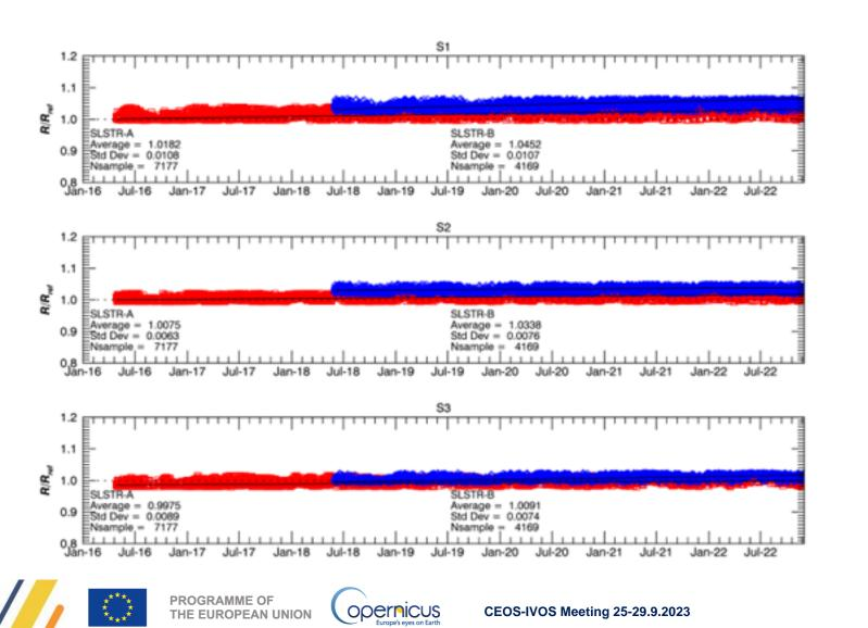
Latest MPC Vicarious Calibration Results for Nadir wrt OLCI (red 3A and blue 3B). Overall the performance is stable with a minor drift that we allow users to correct for.
