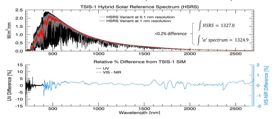
The TSIS-1 HSRS uncertainty is the root-sum-square of the SIM total measurement uncertainty and the 1- $\sigma$  standard deviation of the relative percent difference from the SIM instruments.
