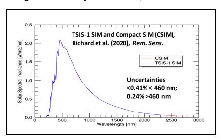
CSIM has an extended spectral range (200~2800 nm) relative to TSIS-1 SIM (200-2400 nm).
