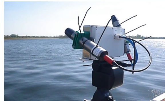
(PANTHYR radiometer System and HYPSTAR® radiometer system. Cable tie spikes are used for bird avoidance).
