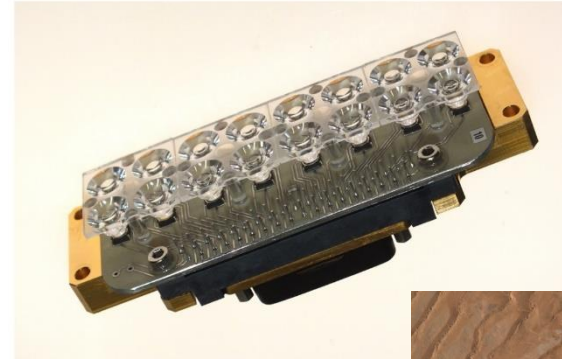
DESI calibration unit 9 LEDs of different wavelengths
