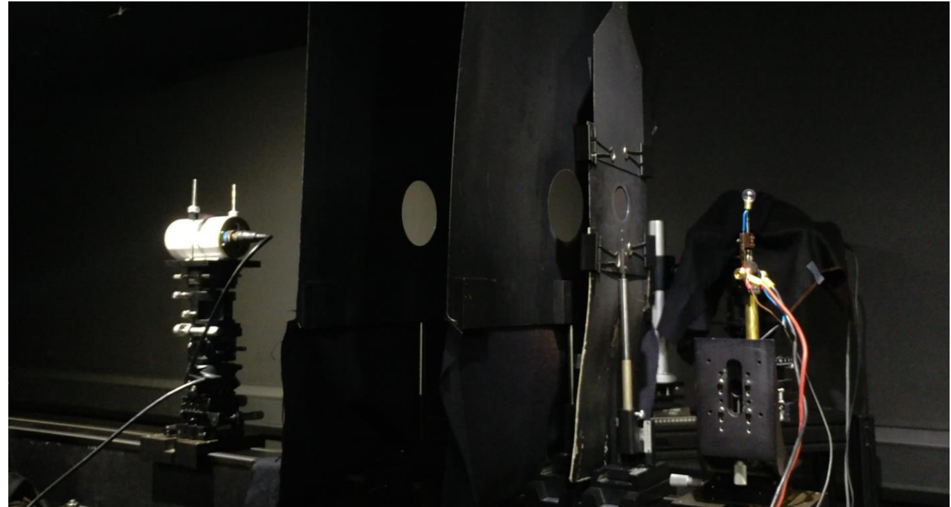
Calibration Setup : irradiance responsivity measurement
