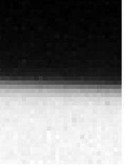
P:\543-S1\Technical\Optical Systems\In Orbit MTF\MTAlong Trackarb2\C2000131\_001\_00\_All\_band centre x: 94 RER: 0.14924257 [%/m] centre y: 128 FWHM [pix]: 4.50900 MTF at: 111.111 [c/mm] 0.063448154 [%] delta x: 30
