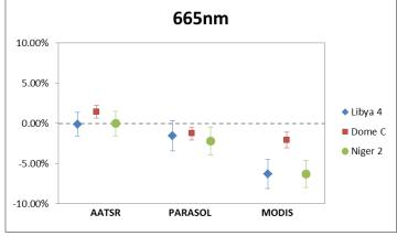
A significant site dependant systematic error due to mismatch in spectral responses between sensors was identified, in particular between MERIS and A-MODIS
