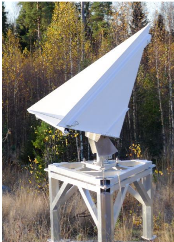
Figure 7: A CR installed at the Finnish Geodetic Observatory Metsähovi in cooperation with DLR. A special tripod base was added to lift the CR above the maximum expected snow level.
