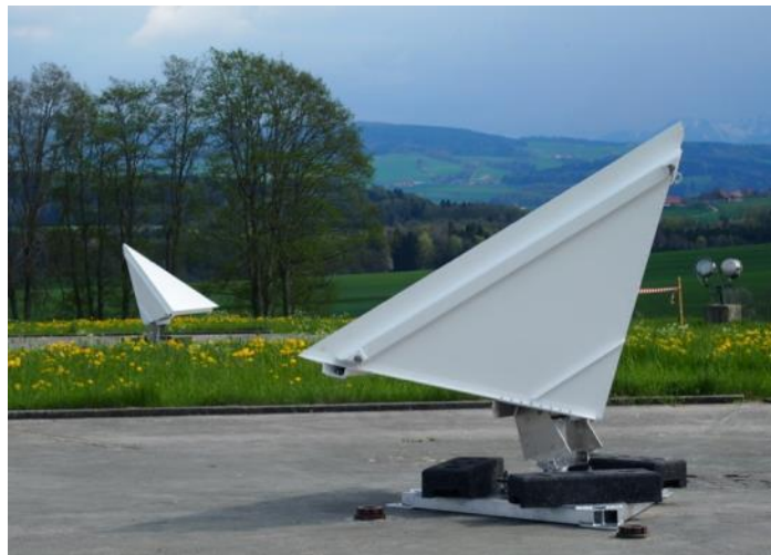
Figure 2: Two UZH 1.5 m corner reflectors in Torny-le-Grand , Switzerland, facing ascending and descending S-1 orbits.
