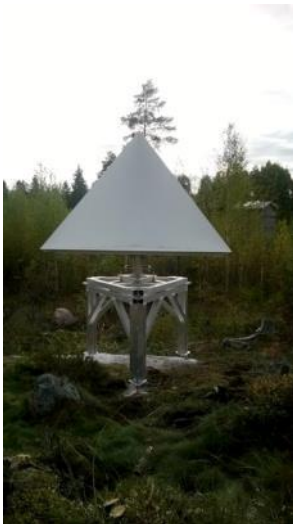
Figure 9: Where applicable, mounting on stable bedrock is a good alternative to a concrete foundation. Example from geodetic observatory Metsähovi , Finland. According to recommendations from the Finnish Geodetic Institute (FGI), the stand of the corner reflector was mounted on the 22mm rods. The holes drilled directly into the bedrock (~40 cm deep) were filled with rock epoxy glue manufactured by Hilti . (© images by FGI)
