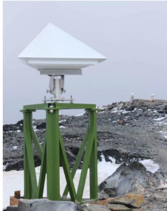
Figure 8: Local weather conditions may require special arrangements. At GARS O’Higgins, Antarctic Peninsula, an additional 1 metre base raised the corner reflector above the winter snow level.
