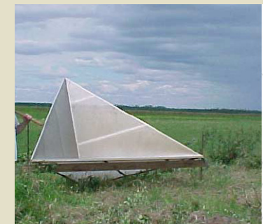
Figure 10. ASAR Transponder set-up at Balikpapan, Indonesia.
