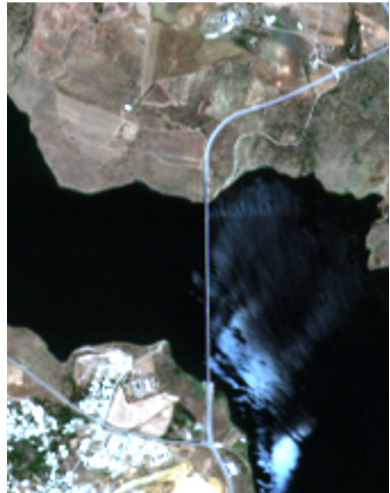
Color image after LOS calibration → Good registration
