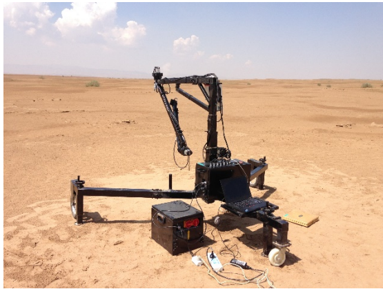
In situ measurement of desert BRF with AOE multi-angle measurement system and SVC field spectrometer
