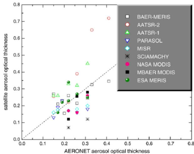
Figure 3: AOT 443: CIMEL versus different satellite sensors [R. 16].
